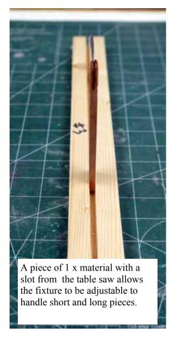
The mount is made from a thin piece of wood with a slot cut in the top for a stiff piece of metal. I cut up a tin can and used that for the mount to the model surface.
