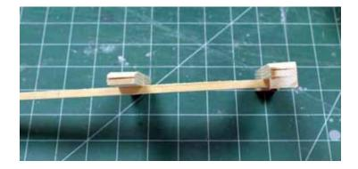
The fixture is simply 2 pieces of wood with slots cut in the ends screwed to a longer stick. Since they are screwed on, they are easily changeable for different models. As you can see in the photo above an extra piece of wood in glued on the right stick to allow the fixture to hold the part a little farther off the table when drying.
