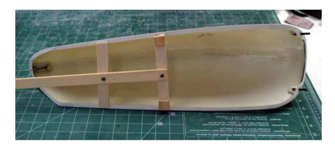
To use, just slide the slots in the end of the cross pieces over the flanges on the chin cowl or canopy. When the part is painted, set the fixture on a flat surface for drying.
