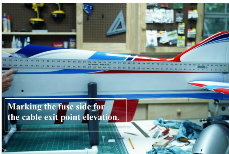
line sets the elevation for the exit holes.
